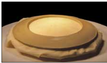
(Figure 3) Clay rim with underlying cloth draped over the glass template
