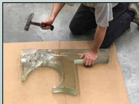
Hammering large fragments of dichro plate glass
