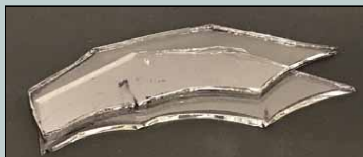
Bat decanter wing blanks created from 3 mm boro plate glass
