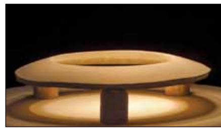
(Figure 4) Drop-out mold on kiln posts
