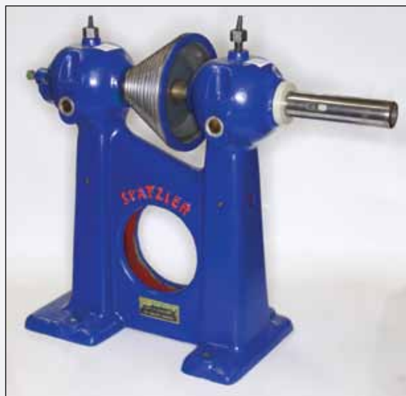
Spatzier produced some of the finest, full-sized engraving lathes, including this refurbished model. Photo courtesy of His Glassworks, www.hisglassworks.com .
