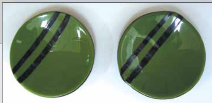
(Figure 1) The edge of the bowl on the left has been cold worked. The shape of the bowl on the right where the two dark stripes end shows the “bulge” from fusing.
