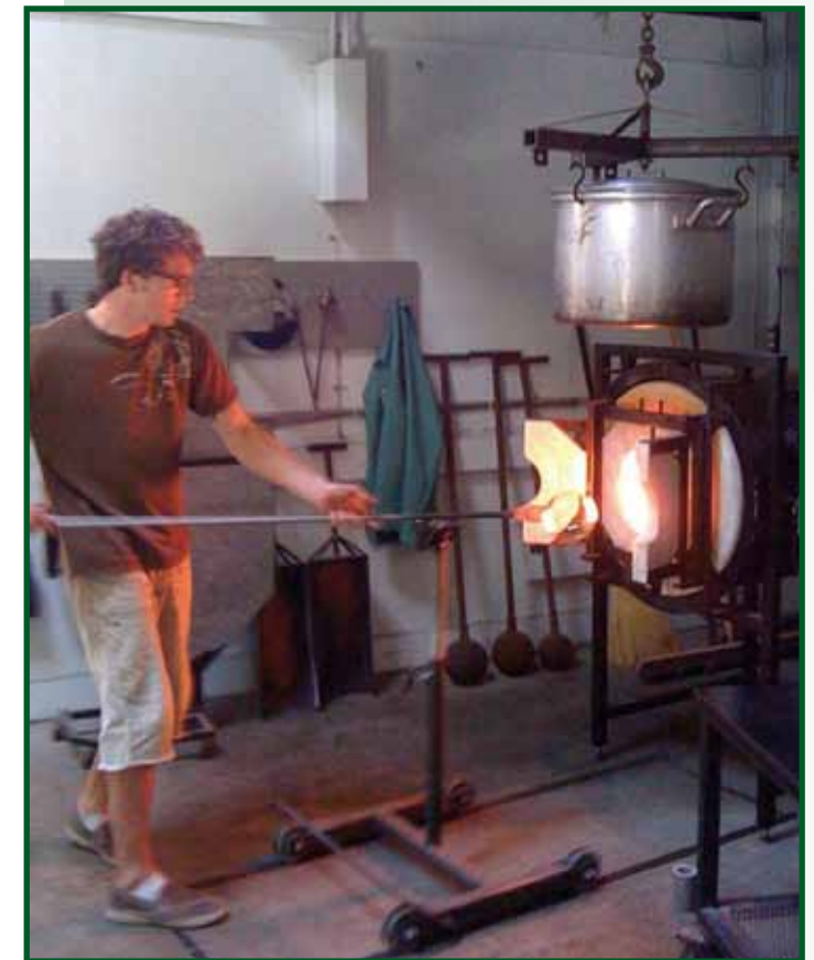
Nick Fruin, STARworks Glass Studio coordinator boiling water while blowing glass in an experiment to see just how much can be done with glory hole waste heat.
